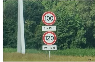
In this road network, the speed limit increases at 19:00.
